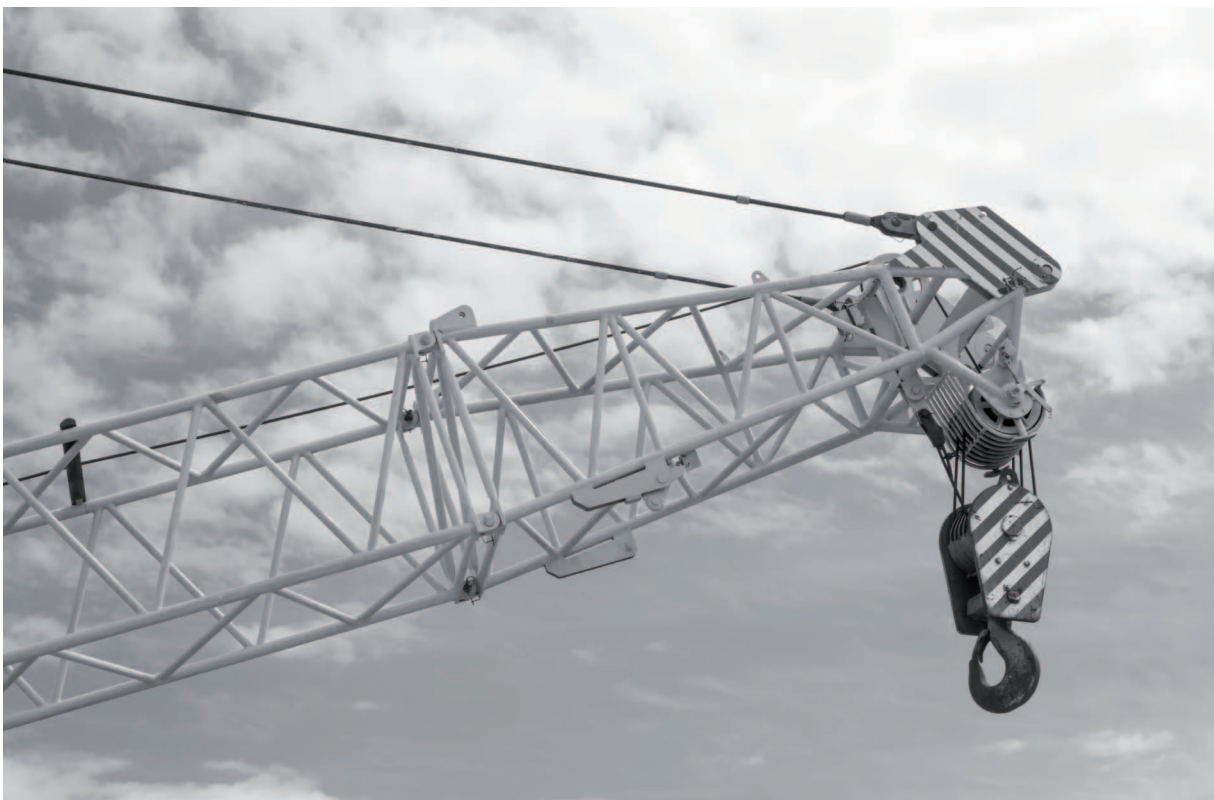
Figure 34 Detail of hoist and boom ropes
