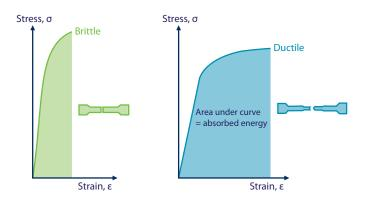
The graph above compares the behaviour of wires with different strengths: the green line represents a brittle trend typical of high strength steel (over 2160 N/mm<sup>2</sup>). The blue line represents the typical trend of lower strength steel (1770 and 1960 N/mm<sup>2</sup>).
