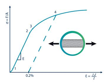
In the first phase of its use (up to point 1), rope shows a certain permanent stretch due to the stabilization of the individual wires. After this step, the trend is basically linear up to the achievement of yield point (points 3 and 4), from which point permanent plastic deformation takes place, until the load reaches the actual rope breaking force.
