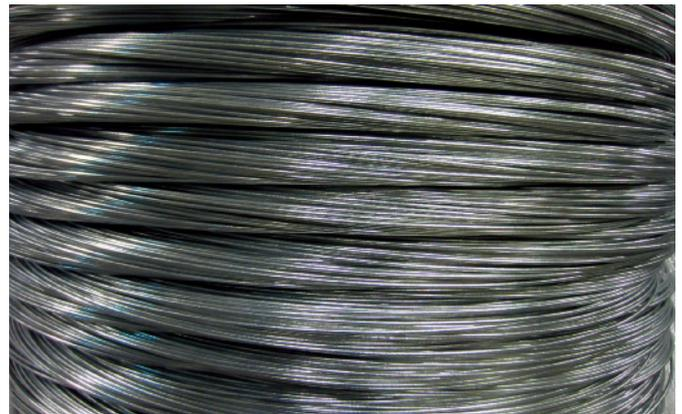
Zinc is applied by a hot dip process in order to avoid hydrogen embrittlement typical of electrochemical plating. Hot dip galvanizing creates a tight connection between zinc and steel, virtually alloying them in one unique entity.
