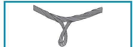
**Protrusion of inner rope**
