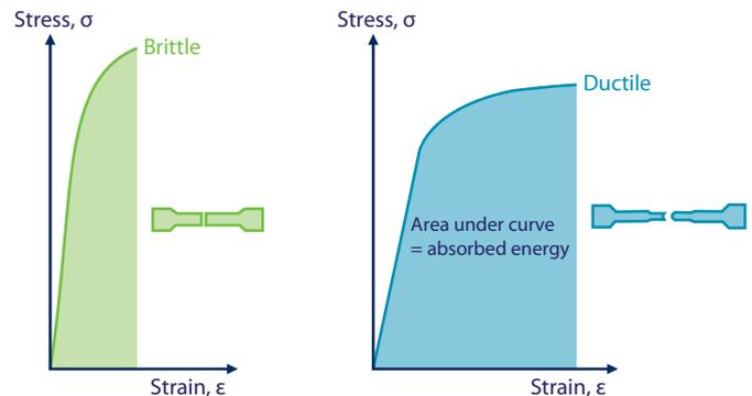
The graph above compares the behaviour of wires with different strengths: the green line represents a brittle trend typical of high strength steel (over 2160 N/mm<sup>2</sup>). The blue line represents the typical trend of lower strength steel (1770 and 1960 N/mm<sup>2</sup>).
