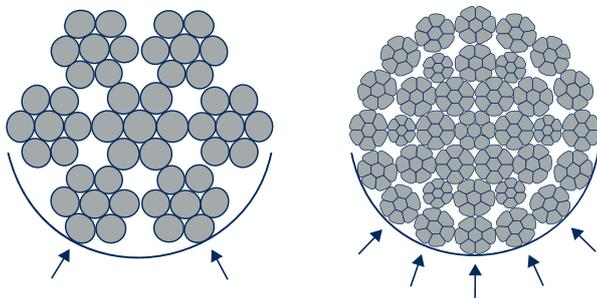
Compacted strands and Lang's lay ropes further extend the contact surface.
