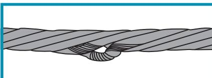
**Strand protrusion or distortion**
